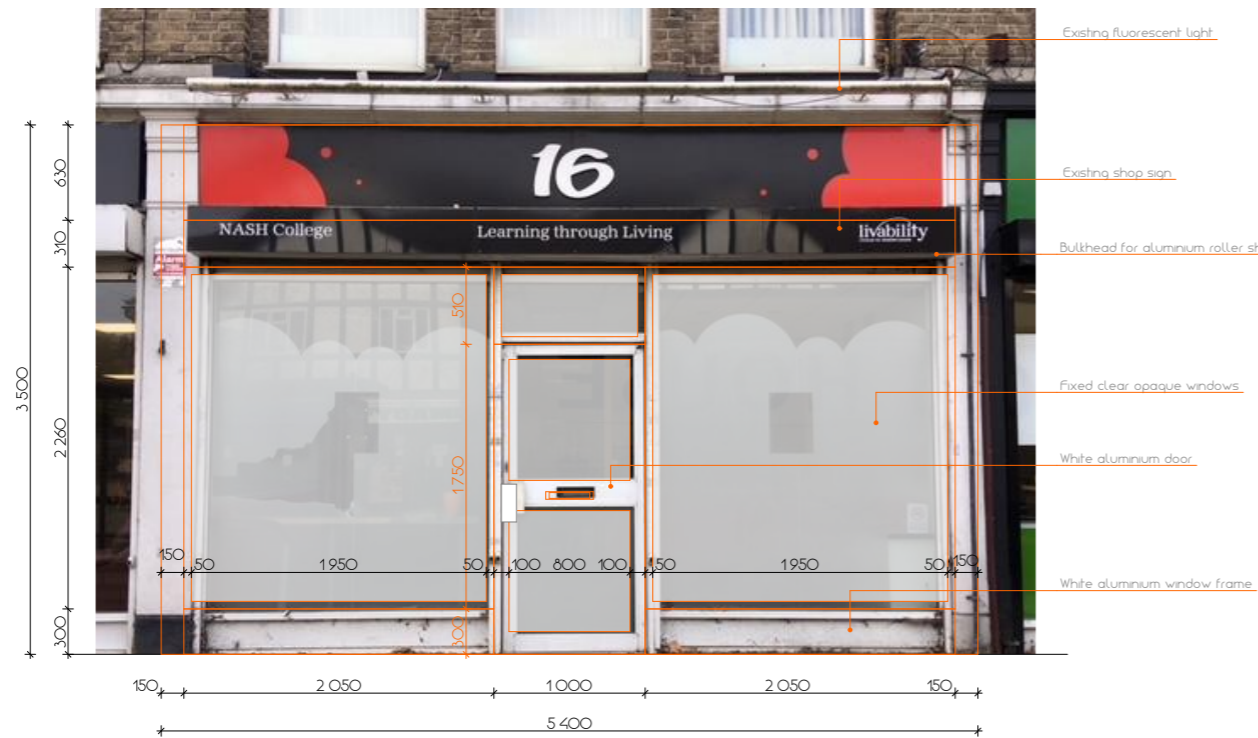
5 ELEVATION, EXISTING SHOP FRONT A-6 SCALE: 1:50
